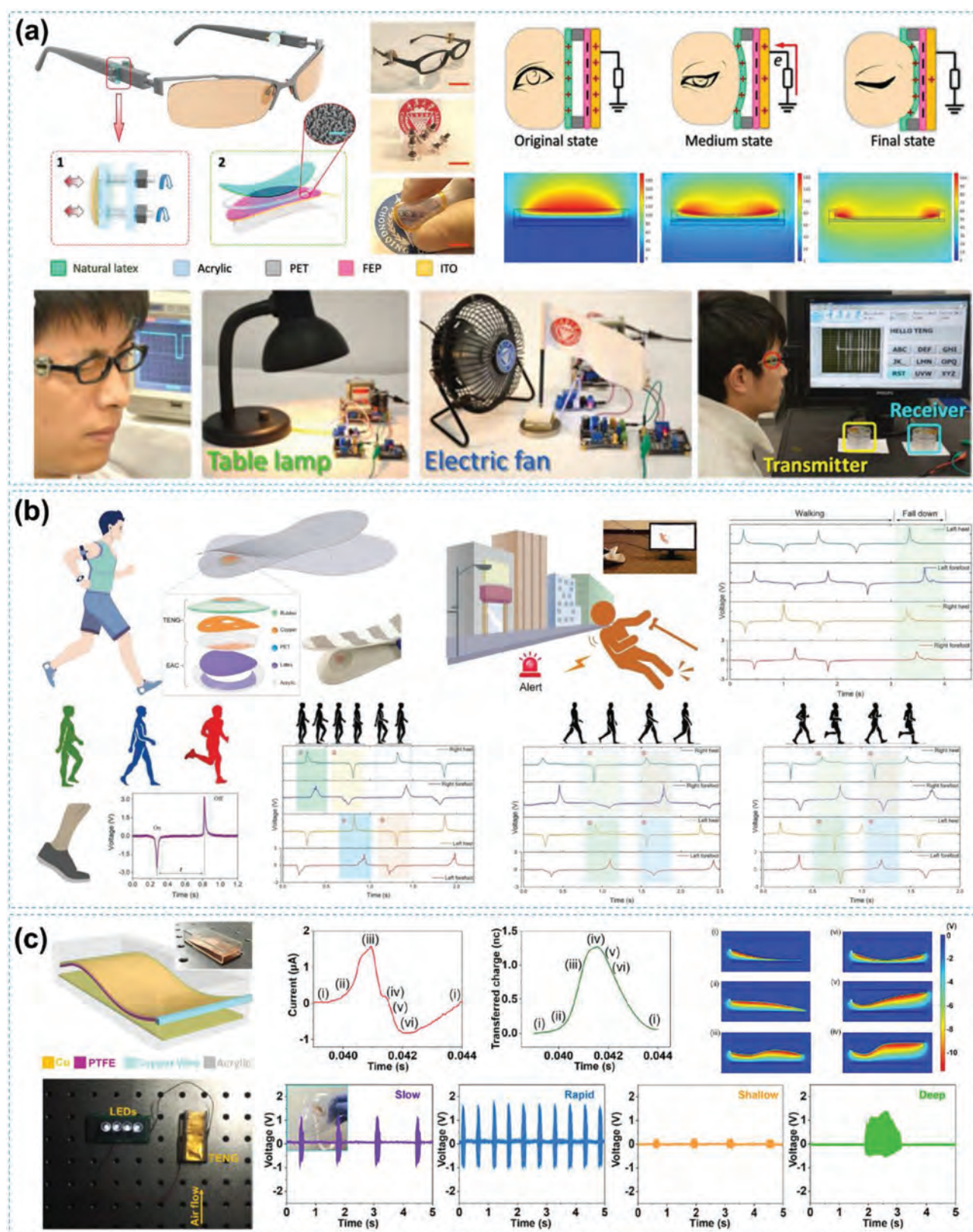
Figure 5. Indirectly wearable TENGs as active sensors for a) A mechnosensational communication system, Reproduced with permission. [45] Copyright 2017, The American Association for the Advancement of Science. b) Monitoring human gait. Reproduced with permission. [46] Copyright 2017, Wiley-VCH. c) Monitoring respiration patterns in real time. Reproduced with permission. [47] Copyright 2018, American Chemical Society.
